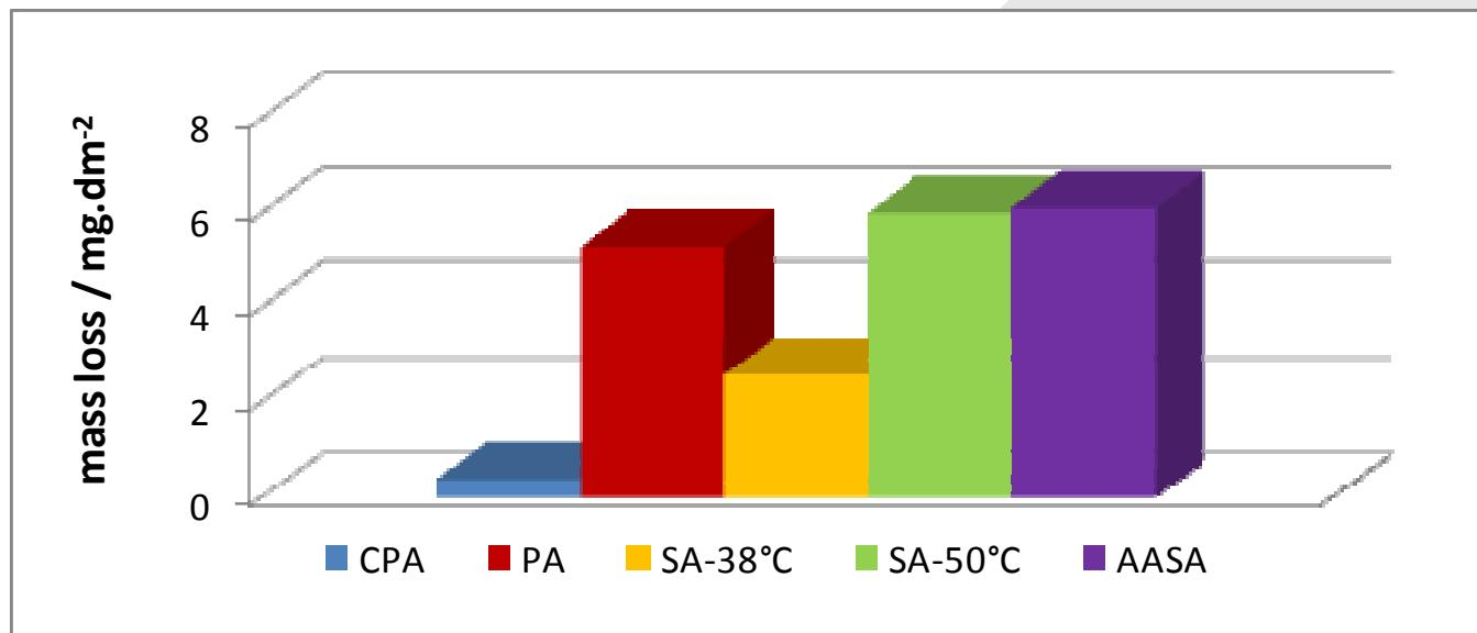
**Influence of increasing the bare aluminium area exposed on the mass loss results of the PA test
