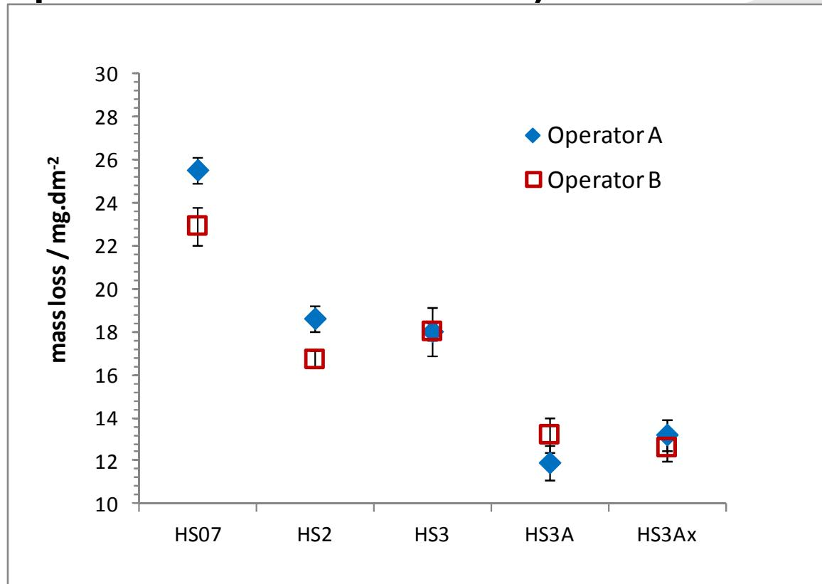
The maximum difference between the two operators mass loss average results was  $2.6 \text{ mg} \cdot \text{dm}^{-2}$ , what is inferior to the reproducibility associated to this method of  $3.6 \text{ mg} \cdot \text{dm}^{-2}$ , estimated in the 2011 QUALANOD's Round Robin Inter-laboratory Test
